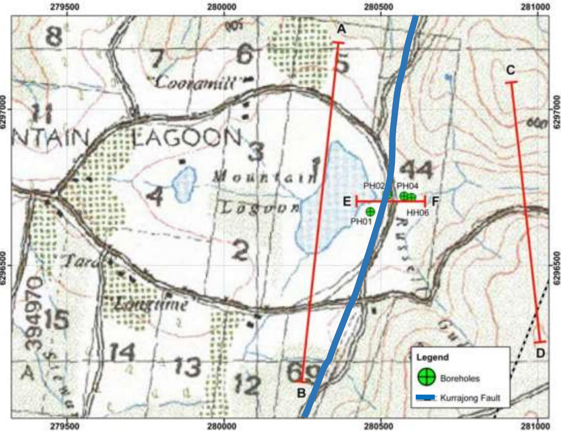
Clark et al drilled bores in a cross-section from E to F ; from the Lagoon and across the Kurrajong Fault
