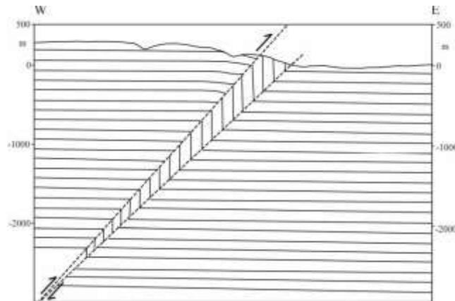
**Figure 3.** *West to east cross section through the Lapstone Structural Complex at the Hawkesbury Lookout (note that stratigraphy is omitted but the surface exposure is in the Hawkesbury Sandstone). Vertical scale = horizontal scale.*
