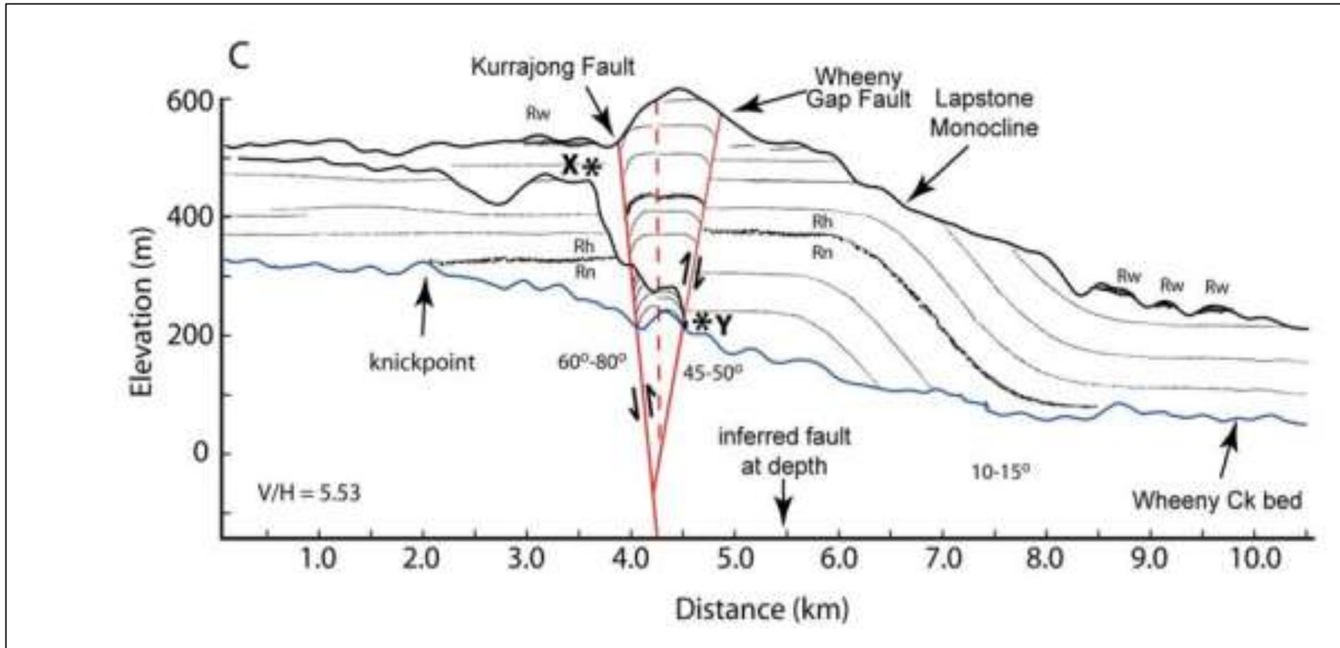
**Figure 4.** Cross Section at Wheeny Gap. Rh =Hawkesbury Sandstone Rn= Narrabeen Group Sandstone. Clark and Rawson 2005.
