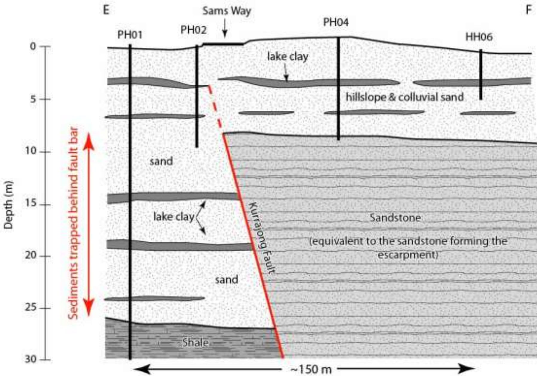
Diagram from Clark et al showing the position and results of their boreholes and the movement on the Fault
